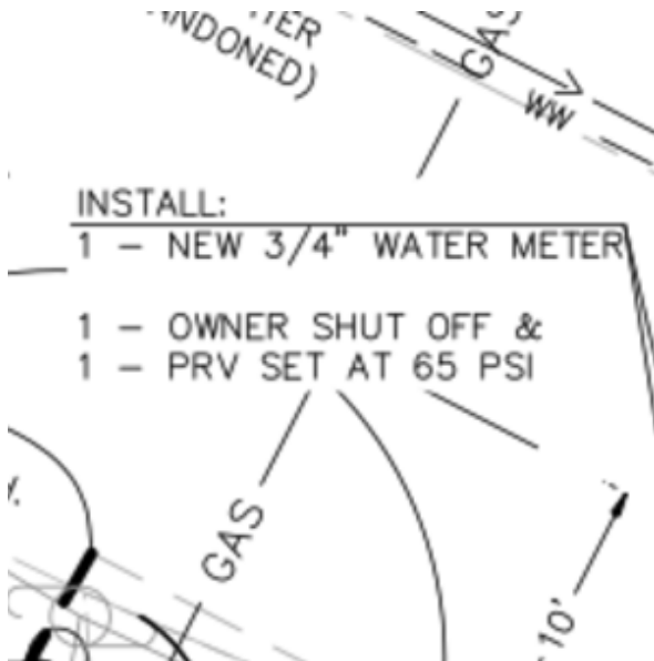
NEW METER, VALVE, PRV REQUIRED
